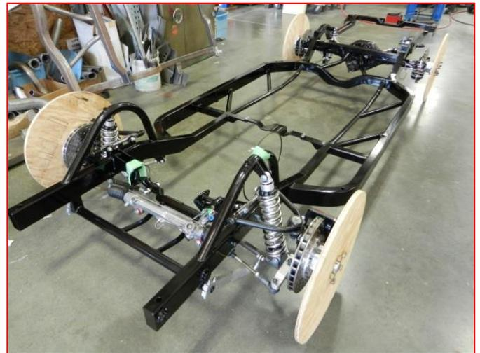
The standard equipment included with each G-Machine chassis is: 6-piston billet calipers with 13-inch rotors, RideTech single-adjustable coilover shocks, a Moser full-floating 9-inch rear end and a Truetrac posi unit, race designed sway bars with billet arms and a power steering rack! The G-Machine chassis design incorporates longer shocks at all four corners than any other chassis which is key to producing optimum ride quality with a low, great looking stance.
