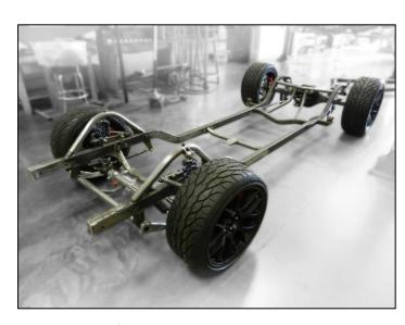
Schwartz G-Machine Chassis incorporates longer shocks at all four corners than any other chassis to improve the overall handling and ride quality of the vehicle
